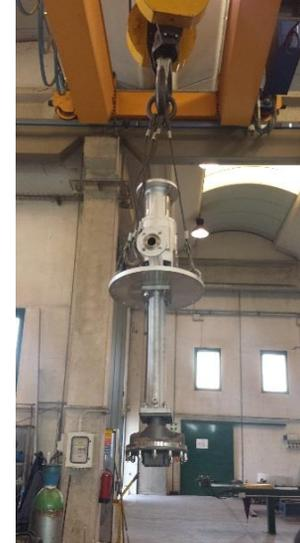
**TWI has been carrying out corrosion tests on stainless steel samples in contaminated molten salts**
