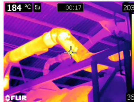
Thermo-mapping of the kiln and the exhaust was conducted by Econotherm using an IR camera to give a thermal analysis of the proposed Smartrec installation area
