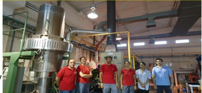
The first tests have been undertaken by ITC-AICE and Econotherm in July and August 2018 to determine the performance of this innovative heat recovery installation under working conditions like those found in ceramic tile industrial kilns.
